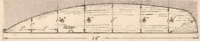
Fig. 4.—Cardboard template for the hull.
