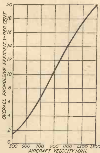
Fig. 21.—Overall propulsive efficiency of ram jet plotted against aircraft velocity.
