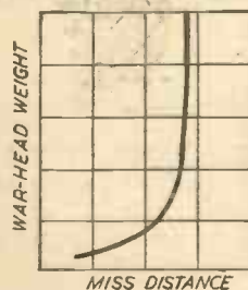
Fig. 10.—Typical relation between war-head weight and miss distance.
