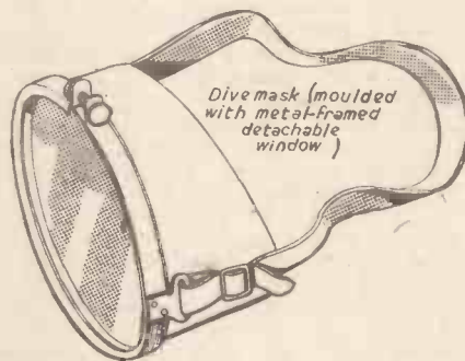
The dive mask used in conjunction with the Aqualung.
