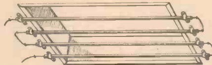
Fig. 6.—A suitable arrangement for safeguarding a skylight by means of a thin insulated wire passed through bars made of split conduit, and connected as shown.
