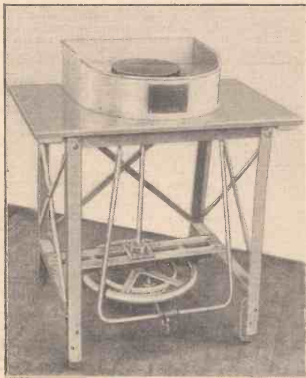
The completed potter's wheel ready for use.
