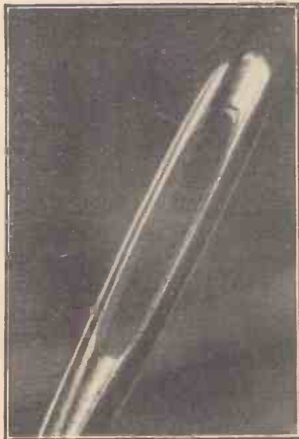
Fig. 9.—Eye of a small sewing needle. 90 secs. at f. 12.5, using Leica. 20 X.
