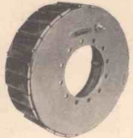
Fig. 6.—Aircraft Drum Brake. Drum brakes are still used on many of the smaller types of aircraft. On this high duty unit the friction lining is riveted in strips transversely across the supporting steel shoes.
