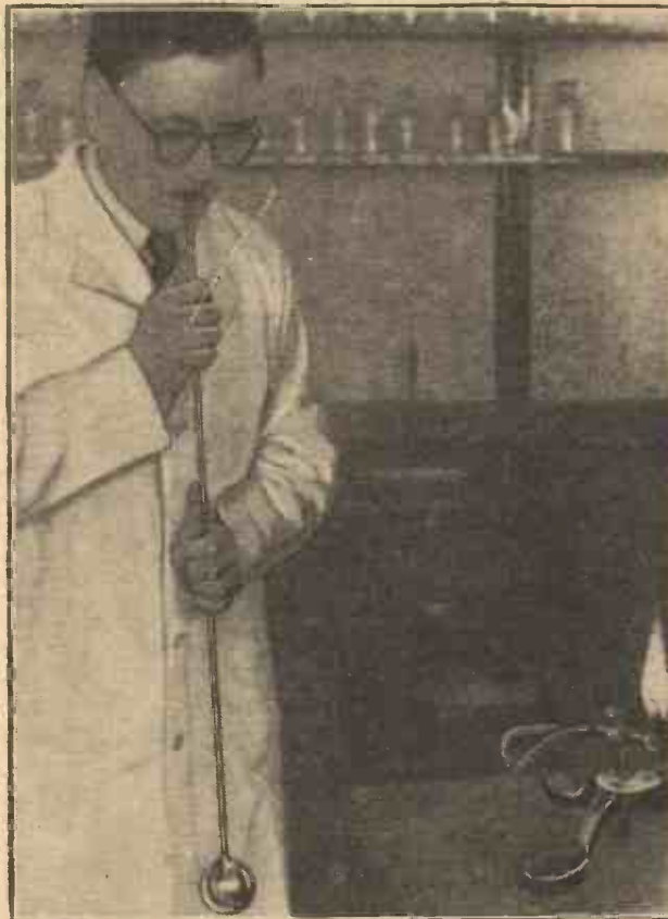
Blowing a bulb. (Note position of the hands. When heating the tube in preparation for blowing, the back of the left hand and the palm of the right hand should be uppermost, so that the tube can be swung quickly into position for blowing.)
