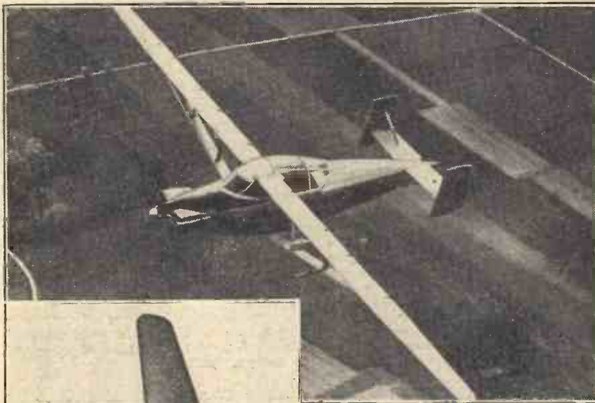
Fig. 1.—Hurel-Dubois HD10 with aspect ratio of 32\frac{1}{2} .
