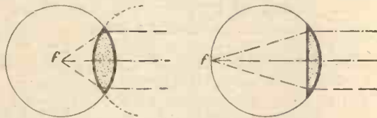
Fig. 2.—Foci of double- and plano-convex lenses of equal radius.
