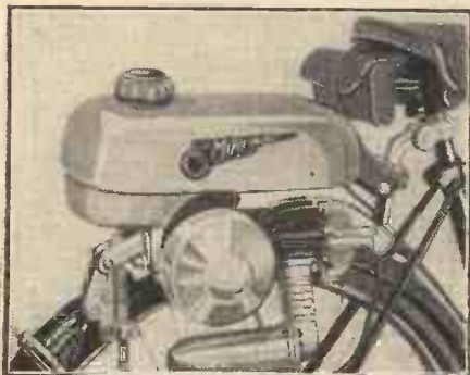
The Mini-Motor, which is a friction-drive on the back wheel.
