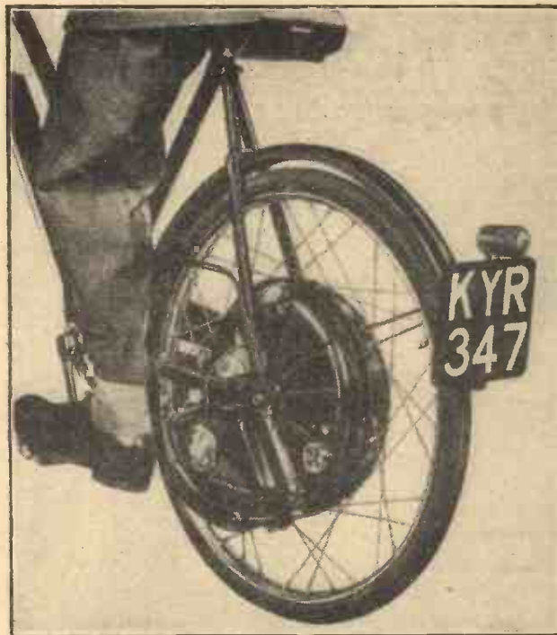
Showing the compact arrangement of the Cyclemaster.
