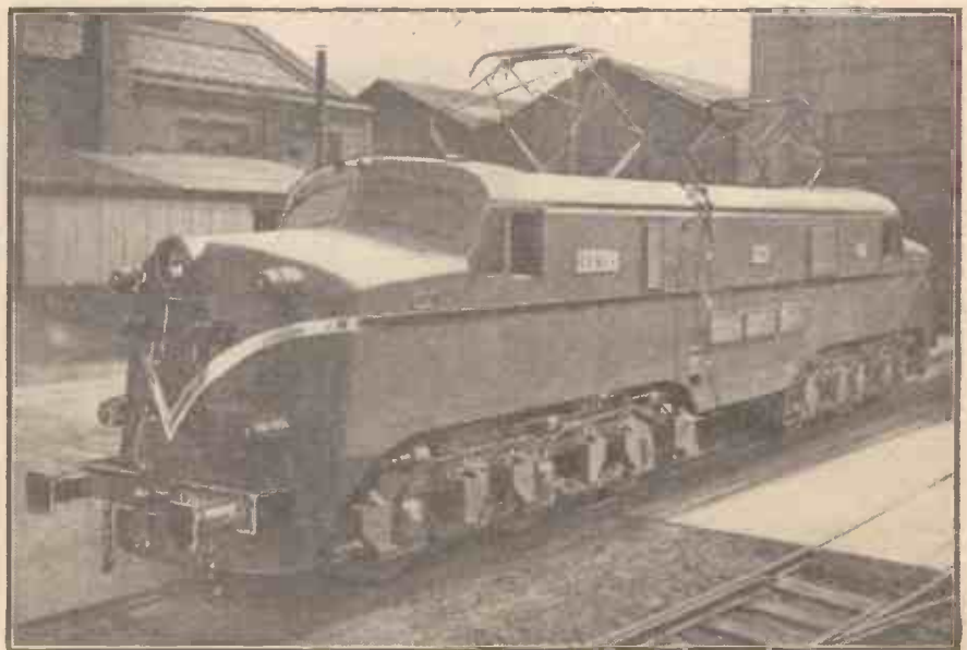
The most powerful electric locomotive yet built in Britain was recently completed at the Vulcan Foundry, Ltd., Newton-le-Willows, Lancashire. It is one of 60 locomotives, each of 3,600 h.p. and weighing 118 tons, ordered by Red Nacional de los Ferrocarriles (The Spanish-National Railways) from the English Electric Company. They are being built jointly by the English Electric Company, Ltd., at Preston, and the Vulcan Foundry, Ltd., at Newton-le-Willows.
