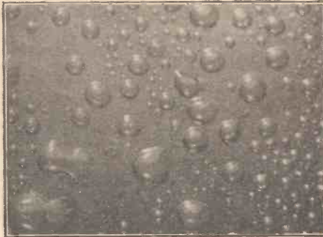
Illustrating the effect of “surface-tension”: what happens to a film of water when it is applied to a greasy plate. The thin layer of water breaks up into innumerable globules, each being drawn up and separated from its neighbours by the forces of surface tension.
