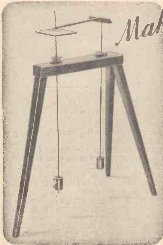
Perspective view of the finished harmonograph.
