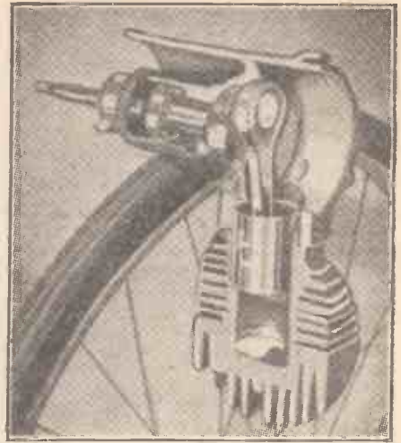
An "exploded" view of the "Power Pak", showing the bearing arrangement of the motor.
