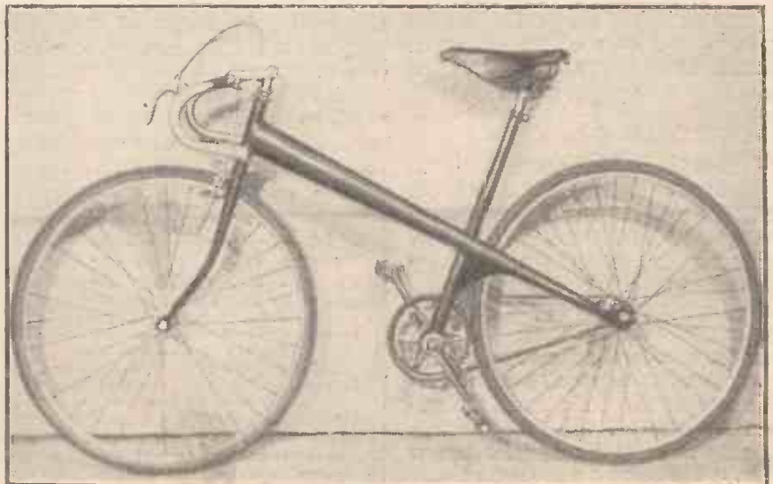
Side view of the new cross-frame bicycle, showing the gusset plate brazed on each side of the frame to give additional strength and rigidity.
