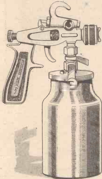
A convenient type of "gun" for spraying the car with enamel or cellulose. It must be used in conjunction with a small air container and a foot-pump.
