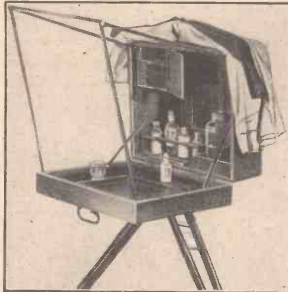
A portable photographic dark-room of the 1870's. On this tripod-supported wooden tray, covered with a dark cloth, the photographic enthusiast coated and developed his plates as and when they were exposed in the camera.
