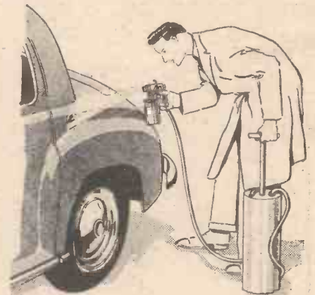
The spraying "gun" must be supplied with air from a small reservoir. Many "guns" now available can be operated from a tyre pump.
