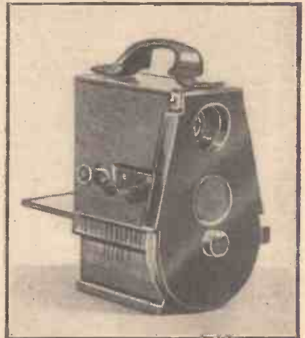
The Brookes-Billcliff miniature camera which accommodates 12 glass plates, each 1\frac{1}{4} in. square. Its shutter was worked by an elastic band. It was made about 1873.
