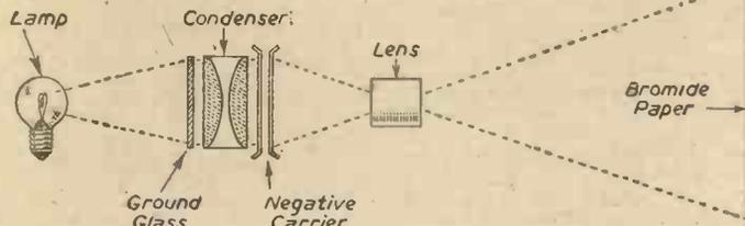
Diagram showing the optical layout for an enlarger.
