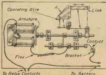
Fig. 3.—The automatic electrically-operated mechanism.
