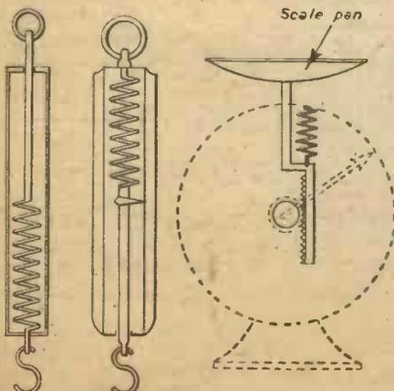
Fig. 7.—Three types of tension spring balances.
