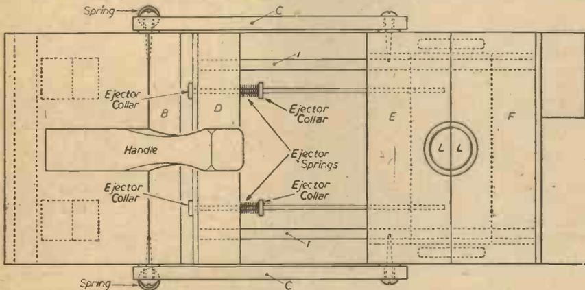
Fig. 2.—Plan view of the machine showing the ejector rods and springs.
