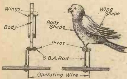
Fig. 4.—Details of the movement for actuating the mechanical "bird."
