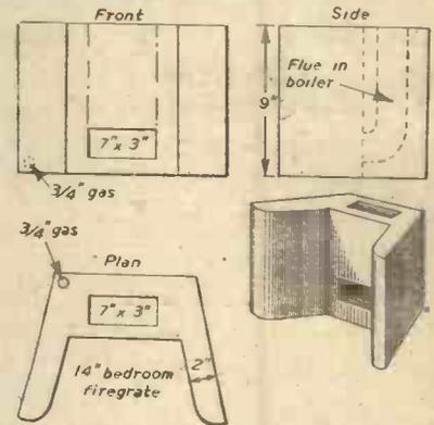
Fig. 2.—Details of the boiler.
