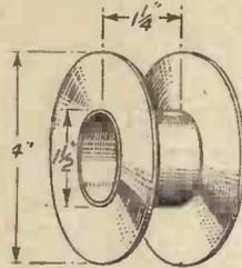
Fig. 3.—One of the coil bobbins.
