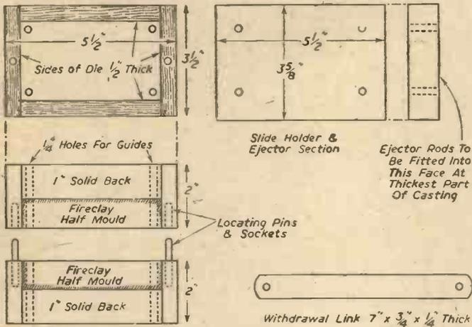
Fig. 4.—Details of die, moulds and withdrawal link.
