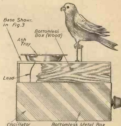
Fig. 5.—Side view of the apparatus, showing the wood and metal casings.
