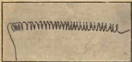
A tiny coil of ruthenium-rich platinum used for thermocouple work.
