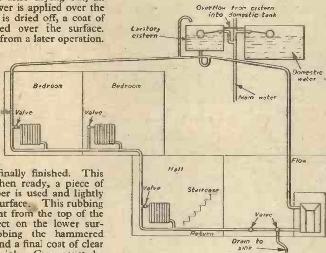
Fig. 1.—Piping layout for a small central-heating system.
