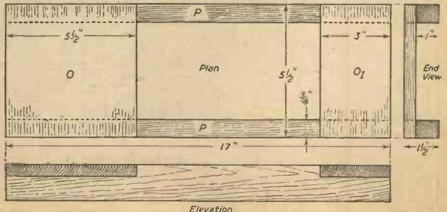
Fig. 3.—Plan and side elevation of the wooden base.
