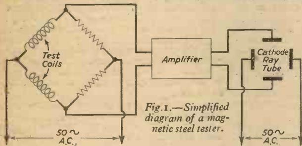
Fig. 1.—Simplified diagram of a magnetic steel tester.
