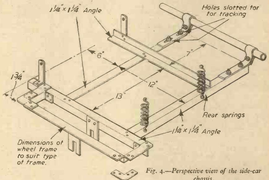
Fig. 4.—Perspective view of the side-car chassis.
