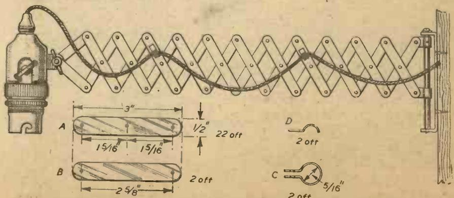
The completed extension bracket, and details of lattice strips and end fittings.
