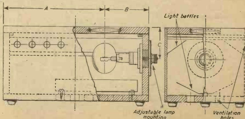
Fig. 4.—General arrangement of lamp housing. Factors governing dimensions: A. Height of draw tube of microscope above base if used as shown in Fig. 2. B. Distance between centre of filament and flange of lampholder plus thickness of inner disc and end of housing. C. Focal length of condensing lens.
