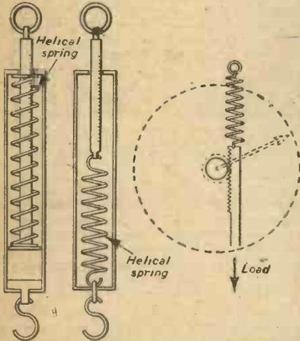
Fig. 1.—(Left) Compression spring balance.
