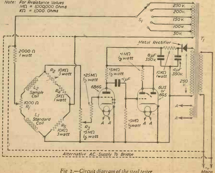
Fig. 2.—Circuit diagram of the steel tester.
