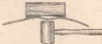
Fig. 5.—A shaped wooden block used as a "dolly" while beating out a dent from inside the wing.
