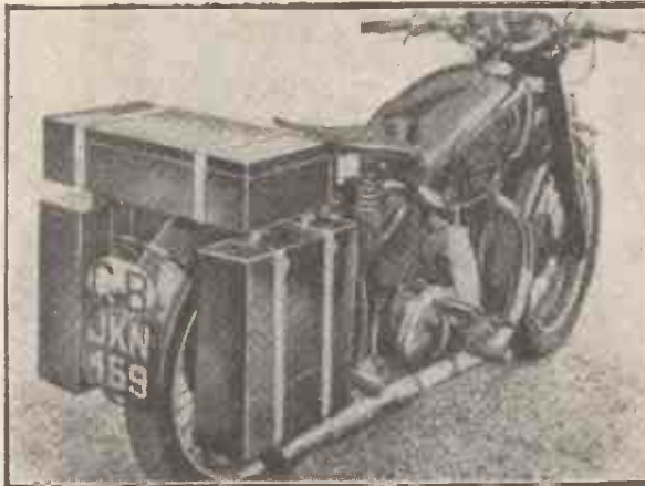
“Craven” pannier equipment of laminated plastic sheet bonded to a wooden framework with a phenolic glue. This equipment has had thousands of miles testing on Continental roads with no deterioration. (By courtesy of Ken Craven.)
