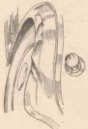
Fig. 7.—A series of dents along the edge of the wing necessitates the use of the shaped wooden blocks.
