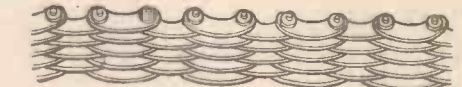
Fig. 93.—Section of "silent" chain. Inset shows how the chain fits the sprocket.
