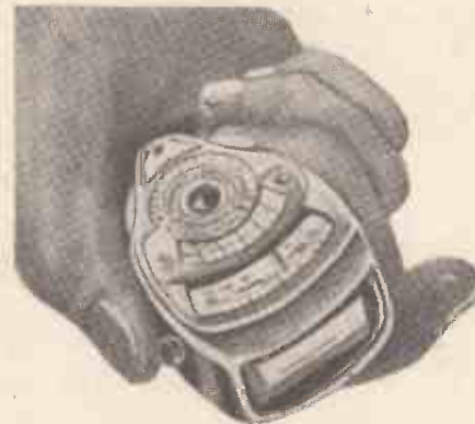
The Pullin photo-electric exposure meter.
