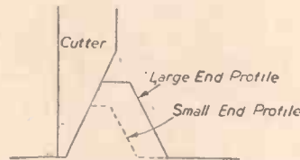
Fig. 62.—Straight-edged cutter fits crown wheel tooth at both ends.
