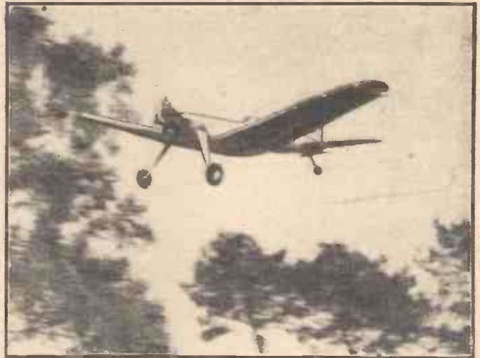
A 7-ft. model diesel-engined aircraft in flight, tethered on the end of control-lines.
