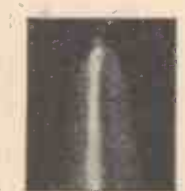
Steel needle after one playing.
