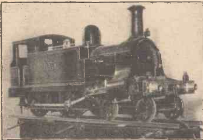
Fig. 1 (Above).—An historic model of a 4-4-0 locomotive, No. 60, of the North London Railway. Built by craftsmen at Bow Works during the Boer War, it is to a scale of 1½ in. to 1 ft.
