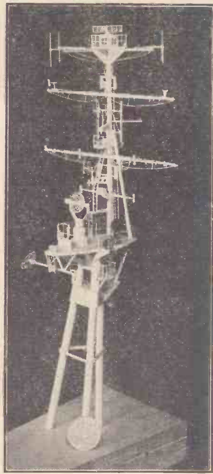
Fig. 5.—Intricate detail model of a battleship tripod mast: the coin at the foot of the model is a half-crown piece.
