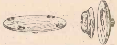
Fig. 39 (left).—Locating pieces glued to faceplate for re-chucking.
