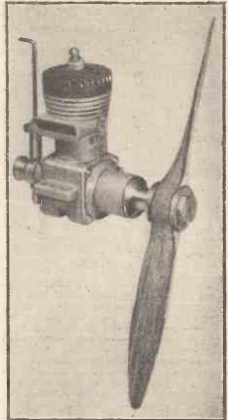
Fig. 10.—The ETA 29 is a new glow-plug engine having a particularly fine performance.
