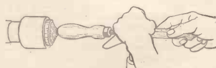
Fig. 31.—Turning a hole in the end of a piece of work.
