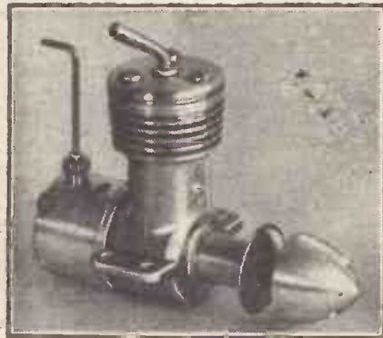
Fig. 6.—The E.D. Mark I "Bee" 1 c.c. diesel engine.
