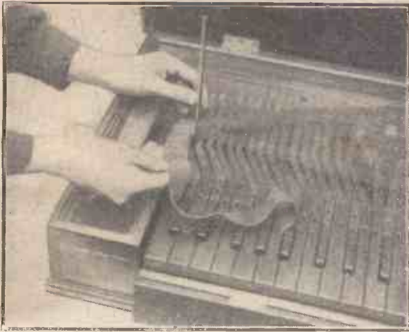
Threading the strip of damping felt through the clavichord strings. The cloth is merely loosely woven under and above alternate wires.
