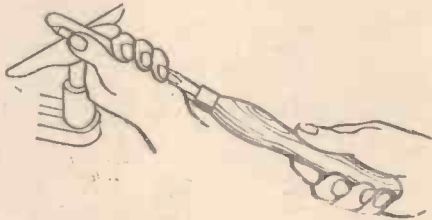
Fig. 16.—The gouge is held at this angle in relation to the work.
