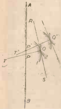
Fig. 21.—Condition for uniform velocity transmission.
