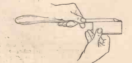
Fig. 19.—The burr inside the gouge is removed by means of an oil stone slip with a rounded edge.
