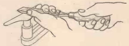
Fig. 17.—How the flat tool is used.
