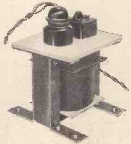
A three-quarter view of the completed transformer.
