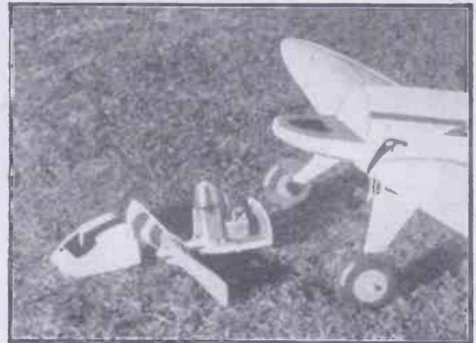
Fig. 20.—This photograph shows the Mills diesel with its beam mounting on the three-ply base with sheet metal stop. The hollow balsa cowling can be seen in front of the engine. The mount is placed on the fuselage ledge and held in position to the fuselage by elastic bands, as can be seen in the next photograph, Fig. 21.
