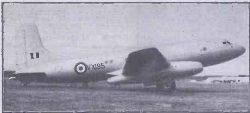
The world's first all-jet four-engined transport aircraft the Tudor VIII, which is powered with four Rolls Royce Nene engines.
