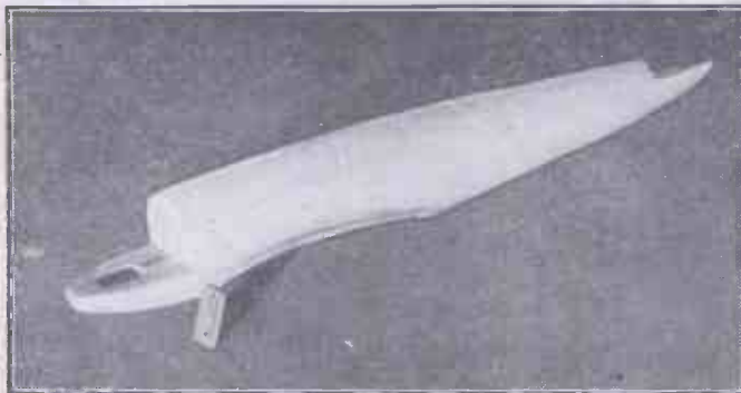
Fig. 18.—The planking has been completed and the fuselage is sanded down smooth.
