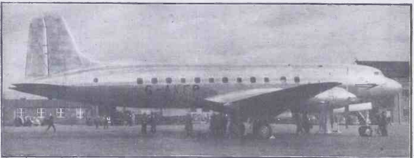
The Handley-Page "Hermes IV" pressurised air-liner with four Bristol "Hercules" engines.
