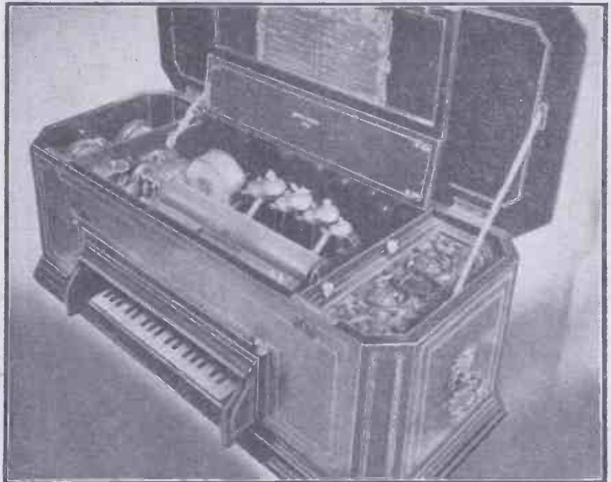
Fig. 2.—Large musical box with two mainsprings and speed regulator. The extreme ends of the comb work the bells, drums and castanets. In the middle are the trackers for the organ which is also connected to the keyboard.
