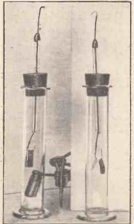
Two electroscopes standing side by side. Both have been given identical electrical charges. The electroscope on the right retains its charge, the gold leaves remaining apart. The electroscope on the left, however, contains a bottle having a fragment of radium barium bromide in it. The rays from this ionise the air within the electroscope, rendering it electrically conductive. The gold leaves thus fail to hold their charge, and they therefore collapse together.
