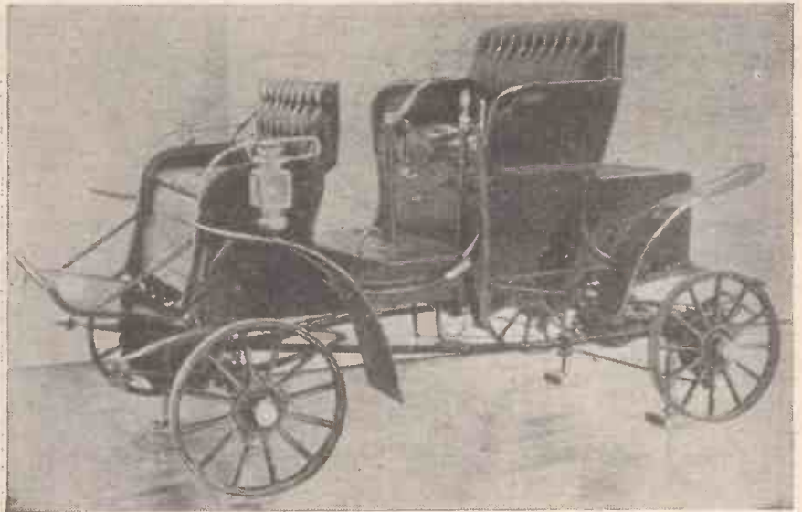
One of Ford's early American competitors. A Stevens-Duryea car of 1904. Note the tiller steering.
