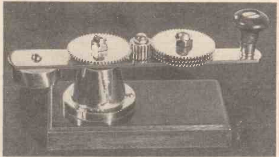
Working model for demonstrating Ferguson's paradox.
