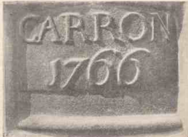
An early specimen of industrial iron. A portion of a cast-iron cylinder made at the famous Carron iron foundry in Scotland.
