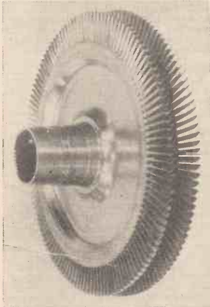
Compressor turbine wheel, showing the double row of blades.
