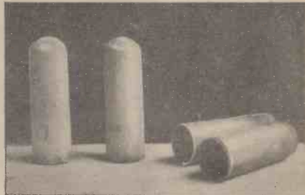
"Soxhelet" thimbles. Cylinders of pure hand-made paper, as utilised in chemical laboratories for the chemical extraction of numerous substances.
