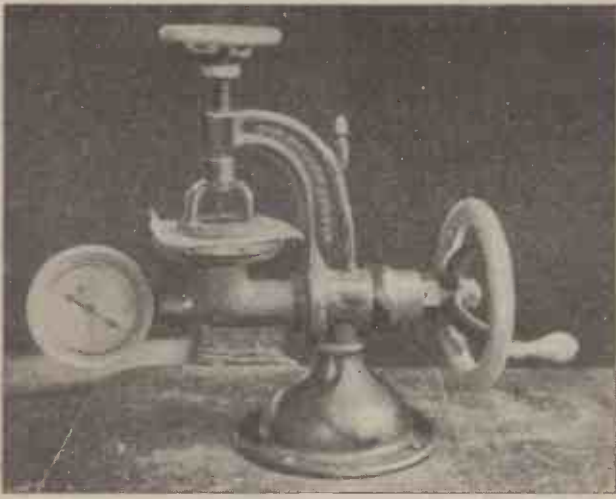
A laboratory paper-testing machine for determining the strength of paper. A fragment of paper is placed within the screw-down clamp and the right-hand wheel is turned, causing an upward stretching of the paper, which ultimately bursts. The bursting strain is recorded by a needle moving over the dial on the left-hand side of the machine.
