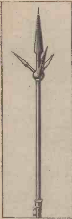
The "business-end" of a modern lightning rod.
