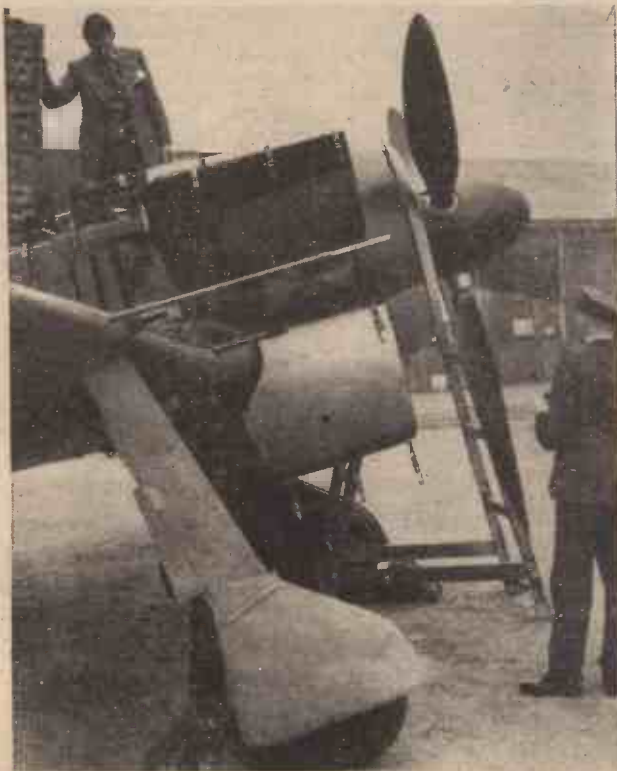
Side view of the front of a FW.190 brought down by a Spitfire on the south coast. The illustration shows the clean lines of engine cowling and two of the 20 mm. cannon guns. On the top of the engine fairing, under the engine cowling, are the two 7.92 mm. machine guns.
