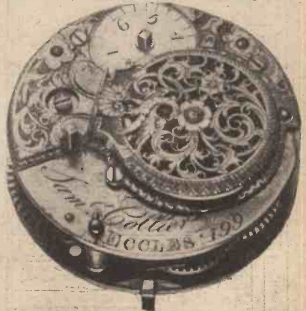
The elaborately ornamented movement of a watch of Earnshaw's day. It was from his efforts to improve the timekeeping of the everyday watch that Earnshaw invented the principle of his chronometer.
