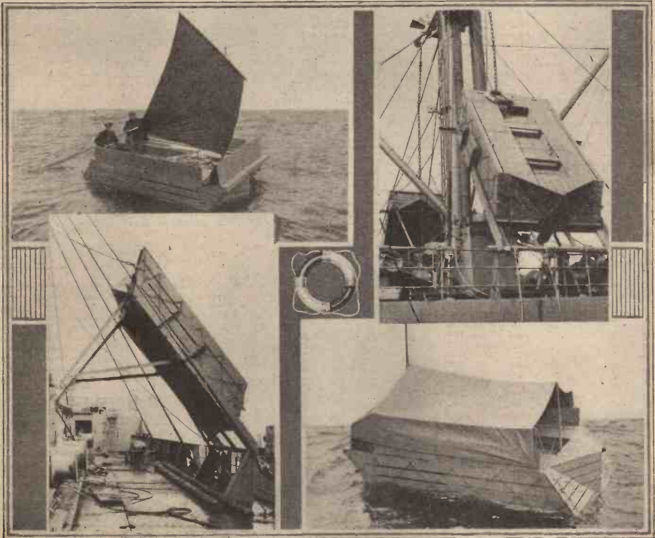
(Top left) Unsinkable Chipchase Patent Lifecraft under sail. (Top right and bottom left) Raft in launching position on board ship. (Bottom right) The lifecraft with awning erected for protection against the weather.
