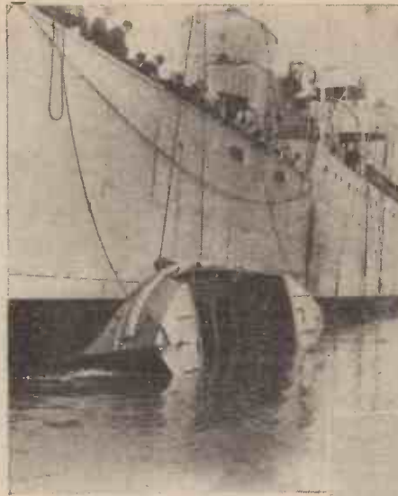
These illustrations show tests being carried out on a self-righting lifeboat designed by Mr. E. H. Lowe, of the Lamport and Holt Line.
