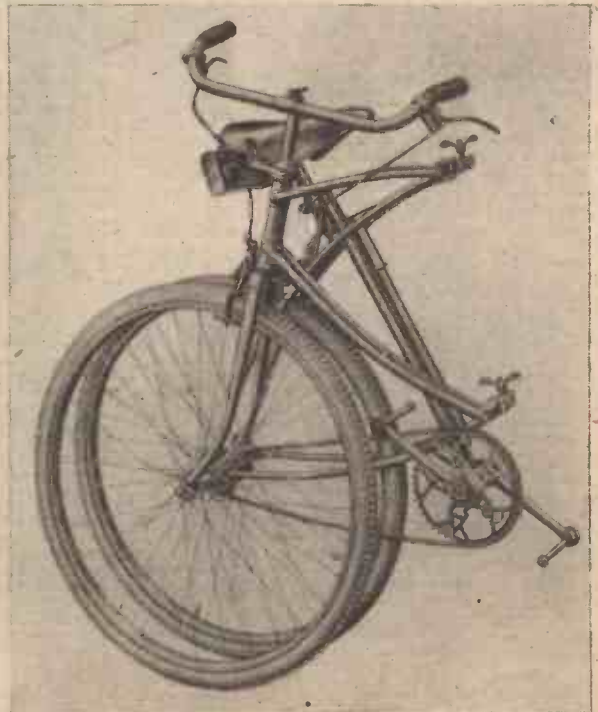
The new B.S.A. folding bicycle ready for the road, and folded ready for transport.
