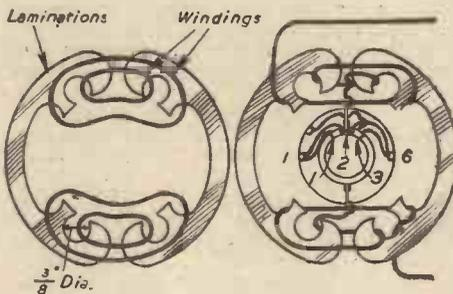
Field circuit and diagram of windings for a converted D.C. motor for driving an electric drill.
