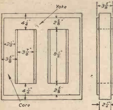
Fig. 2.—Core dimensions for 23 k.V.A. transformer.
