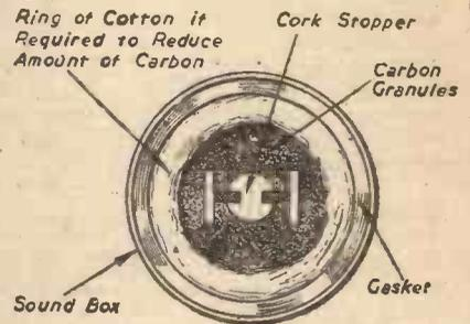
Fig. 2.—Front view of sound-box with diaphragm removed.
