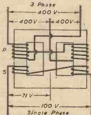
Fig. 5.—Tee connection for three-phase to single-phase conversion.
