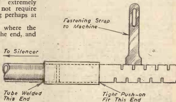
Fig. 1.—Showing method adopted to simplify the removal and cleaning of a blanked-end exhaust pipe.
