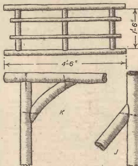
Fig. 9.—How the roof of the garden arch is formed, and details of some of the joints.
