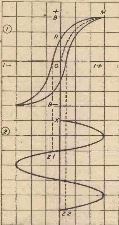
Curves indicating cycle of magnetisation of iron by alternating current.
