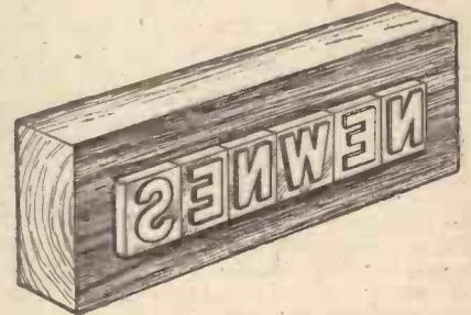
Fig. 4.—The letters should be attached to the rubber by means of rubber solution.
