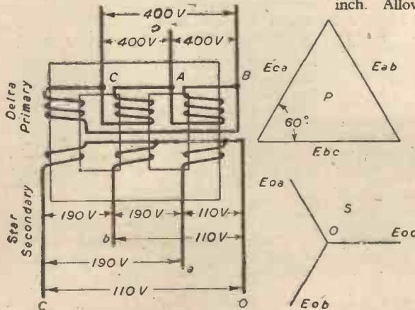
Fig. 3.—Connections and voltage relations in three-phase delta-star step-down transformer.
