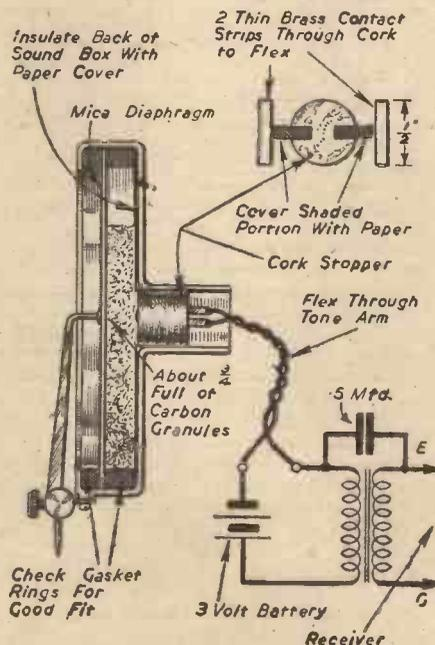
Fig. 1.—Sectional details and circuit diagram of a sound-box pick-up.
