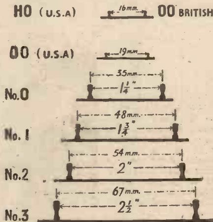
Dimensioned drawing of the different model railway gauges mentioned in the article.
