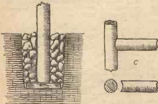
Fig. 2.—(Left) Method of embedding posts in the ground, and (right) how horizontal members are joined to uprights.
