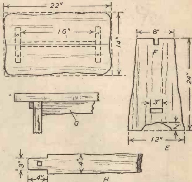
Fig. 7.—Constructional details of the garden table described in the text.
