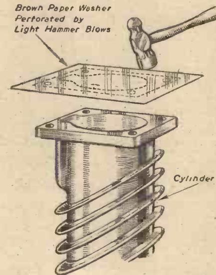
Fig. 3.—Method of making a cylinder-base washer.
