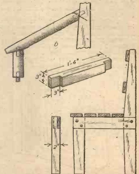
Fig. 5.—Side view of garden seat, and details of arm rest and seat rail.
