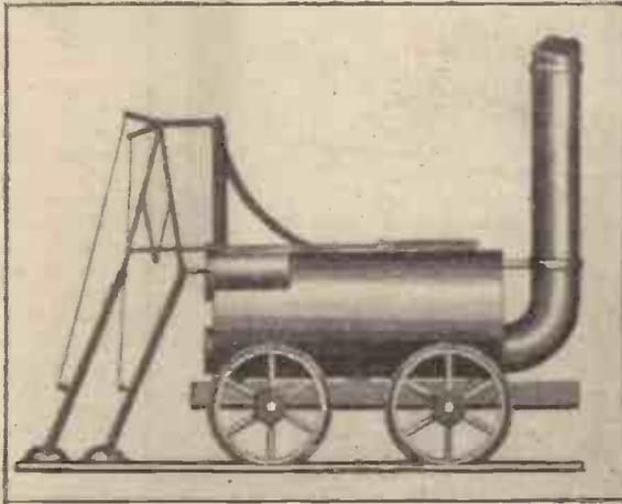
Brunton's "Legged Locomotive"—the "Mechanical Traveller."
