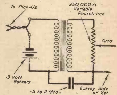
Fig. 3.—Transformer diagram of connections showing external volume control.
