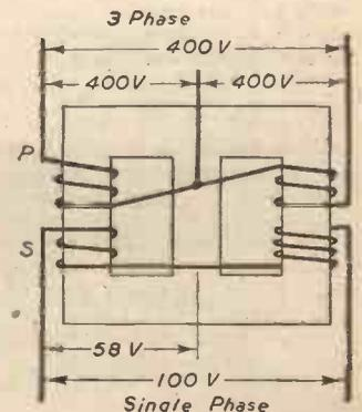
Fig. 4.—Open delta connection for three-phase, to single-phase conversion.
