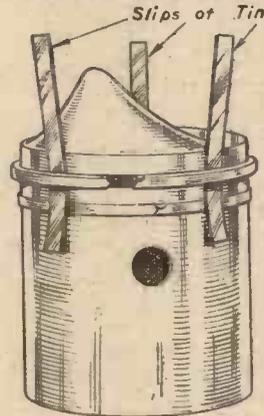
Fig. 2.—Illustrating the method of removing piston rings by three slips of tin.
