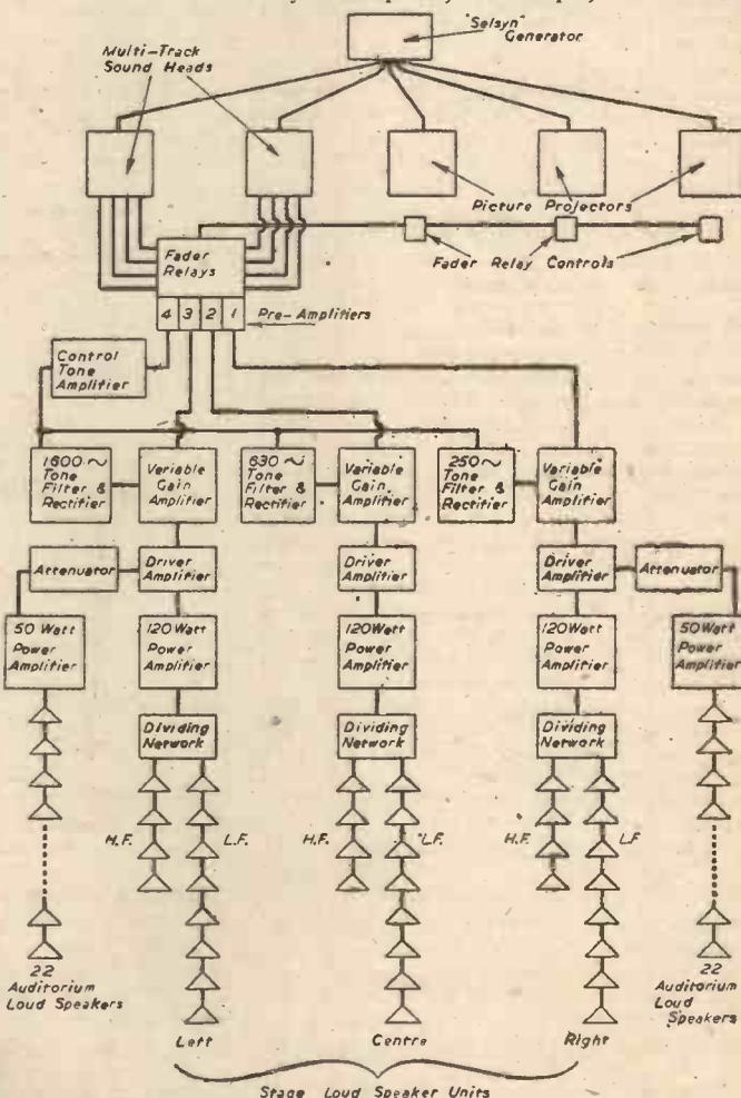
Stereophonic sound recording reproduction, which is discussed in this article, has been successfully demonstrated in America, by R.C.A. Photophone engineers, when reproducing the original sound tracks for Walt Disney's film "Fantasia." A schematic diagram of the amplifier-loudspeaker equipment used is shown herewith.
