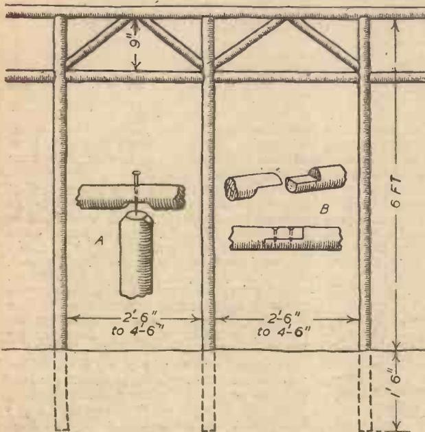
Fig. 1.—A simple rustic pergola, and details of joints.
