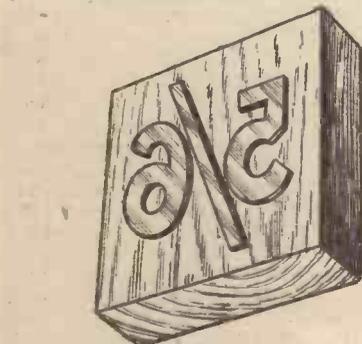
Fig. 5.—Larger stamps, as shown, can be cut from sheet rubber and glued to a wooden base.
