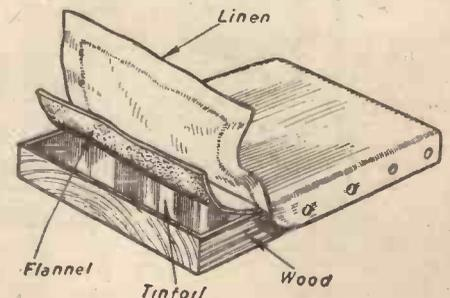
Fig. 7.—Method of constructing the inking pad.
