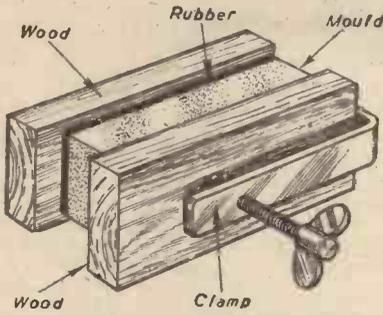
Fig. 2.—How the rubber for the stamp is prepared.
