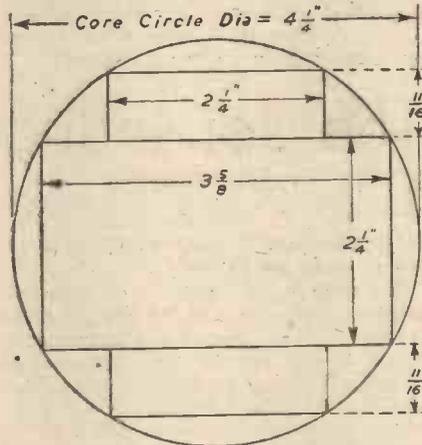
Fig. 1.—Core section for 23 k.V.A. transformer.
