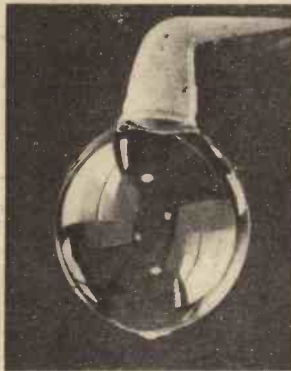
Here the bubble has become more spherical. Most of its surplus material has been drawn up from its lower end in consequence of the stretching of its sides. Only a small amount of surplus material is visible at the lower end of the bubble.
