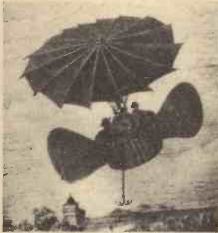
One of the many early suggestions for a hand-operated flying machine—which principle Sir George Cayley showed to be impossible.
