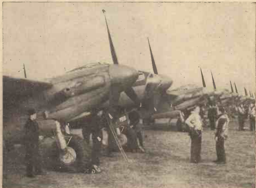
Mosquitoes and their pilots standing by in readiness for a take-off for a raid. This twin-engined R.A.F. reconnaissance bomber is of wooden construction, and has two Rolls Royce engines. Its armament consists of four 20 mm. cannon, and four .303-machine guns.
