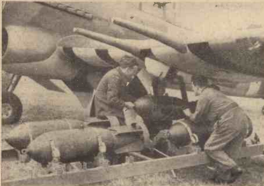
Bombing up a Typhoon fighter bomber. This single-seater day and night fighter is powered by a 2,400 h.p. Napier Sabre engine. Two types of Typhoon are now in service, MK1A, equipped with twelve .303 machine guns, and MK1B, with four 20 mm. cannon. The muzzles of two of these formidable weapons can be clearly seen in the illustration.
