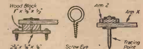
Fig. 3.—The wood block for clamp. Fig. 4.—How the tracing point is made. Fig. 5.—An ordinary screw-eye is point is made. graph to the used where drawing board. show in Fig. 1.
