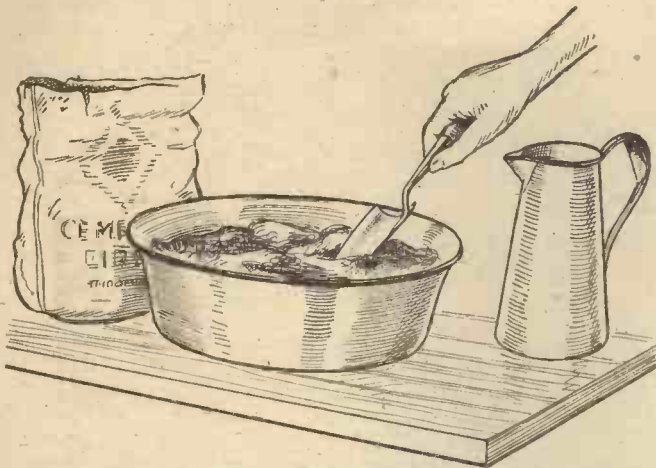
Fig. 2.—Mixing the coal dust and cement in an old bowl.
