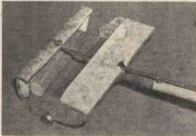
This device, invented by an American, is for picking up incendiary bombs and trapping them in a metal container.
