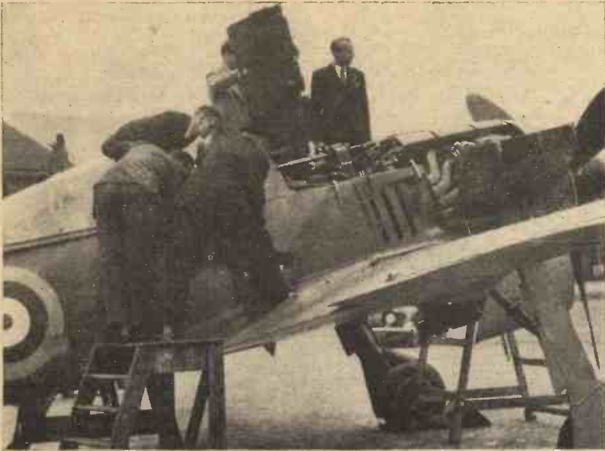
Experts examining the controls in the cockpit of the F.W. 190. The well-balanced B.M.W. 1,600 h.p. engine can be seen, also the two 7.92 mm. machine guns, mounted on the top of the engine.
