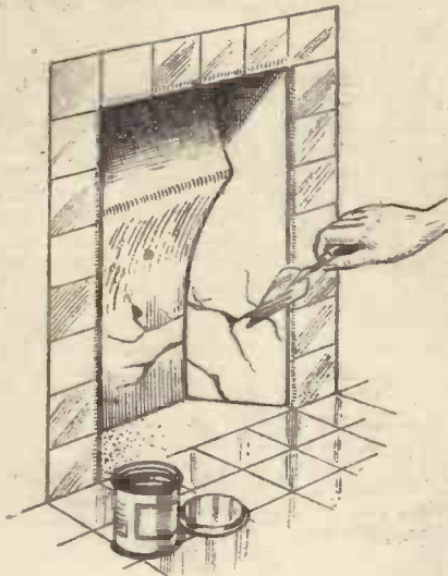
Fig. 1.—Using plastic cement for repairing the back and sides of a fireplace.
