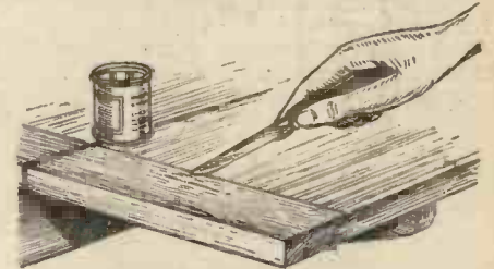
Fig. 7.—Using plastic wood for filling cracks in furniture.
