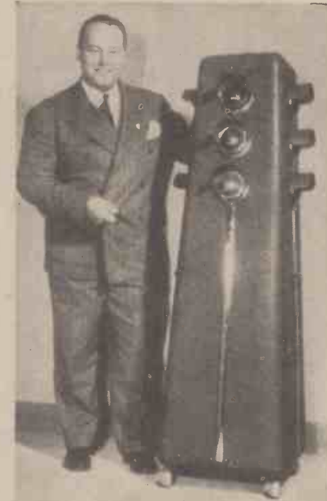
A portable automatic electric traffic signal operated by a 6-volt storage battery. The inventor, G. W. Walker, of Detroit, U.S.A. is here seen with the new unit.
