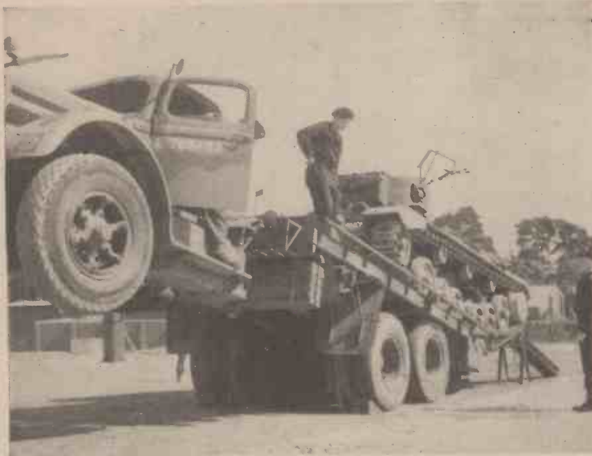
A demonstration of the usefulness of a "Tank Transporter" was recently given in the South Eastern Command. The Transport—an American "White" Tank Lorry—weighs over 30 tons when fully loaded. It has a 130 h.p. engine and is larger than any other road vehicle in Great Britain. In the illustration, the bonnet of the "White" Lorry is seen nosing the air as a "Valentine" climbs up the runners
