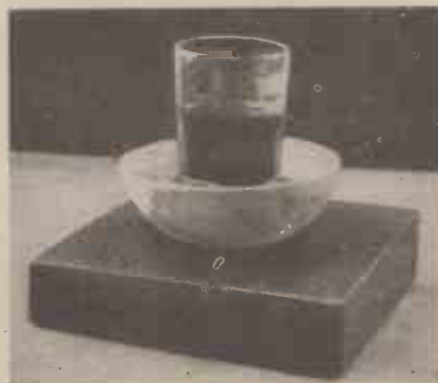
"Dialyzing" a solution of iron hydroxide—a simple process of colloid chemistry
