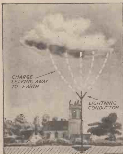
Fig. 3. Lightning conductor tends to move cloud charge leak away to earth
