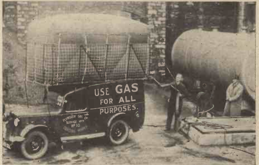
The first gas fuel car in the West Country being filled at the Plymouth city gas works in 1939.
