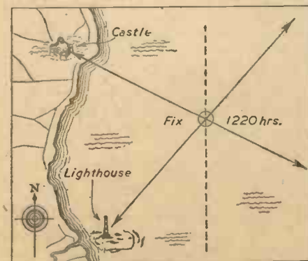
Fig. 6. How the intersection of the bearings gives an aircraft's position.
