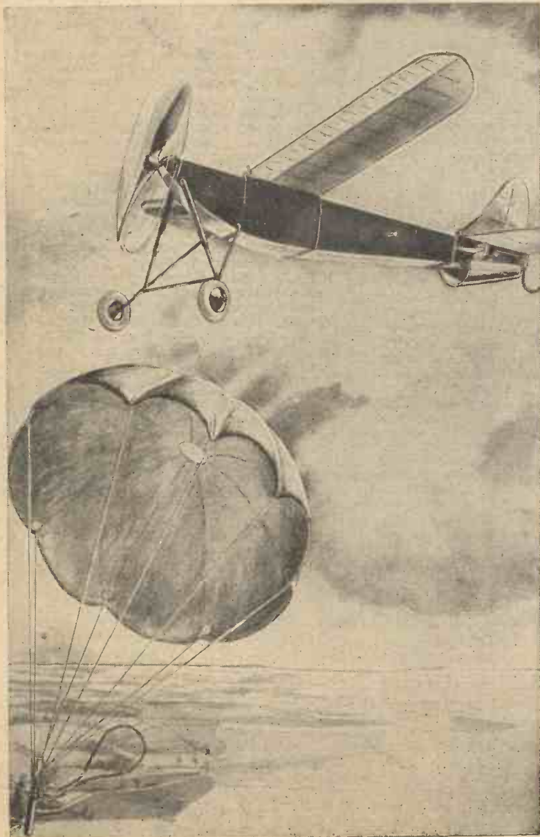
AIRCRAFT AT TOP OF CLIMB. REDUCED MOTOR TENSION ALLOWS CATAPULT TO DRAW OUT METAL PEG. Fig. 3
