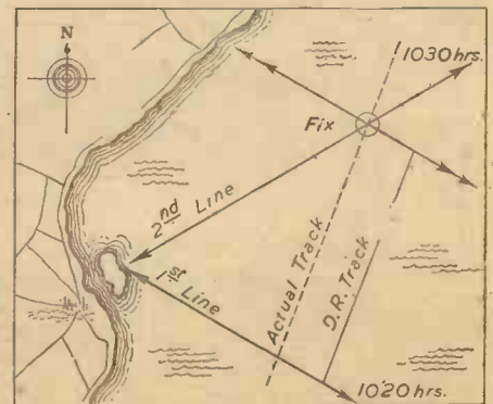
Fig. 7. How the dead-reckoning track is plotted.
