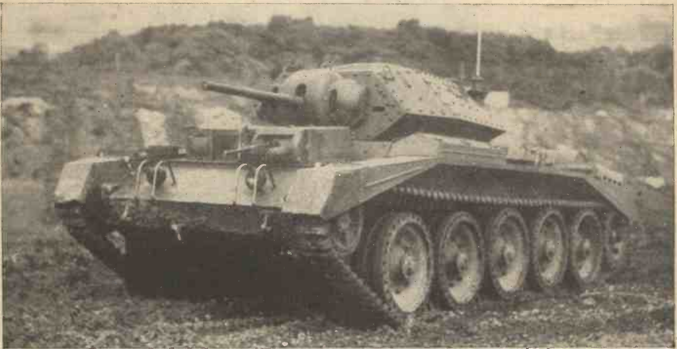
The "Crusader," an 18-ton cruiser tank which is one of the fastest tanks in the world. It has the speed and easy handling of a light car
