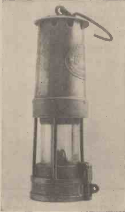
A Davy safety lamp as used in mines at the present day.
