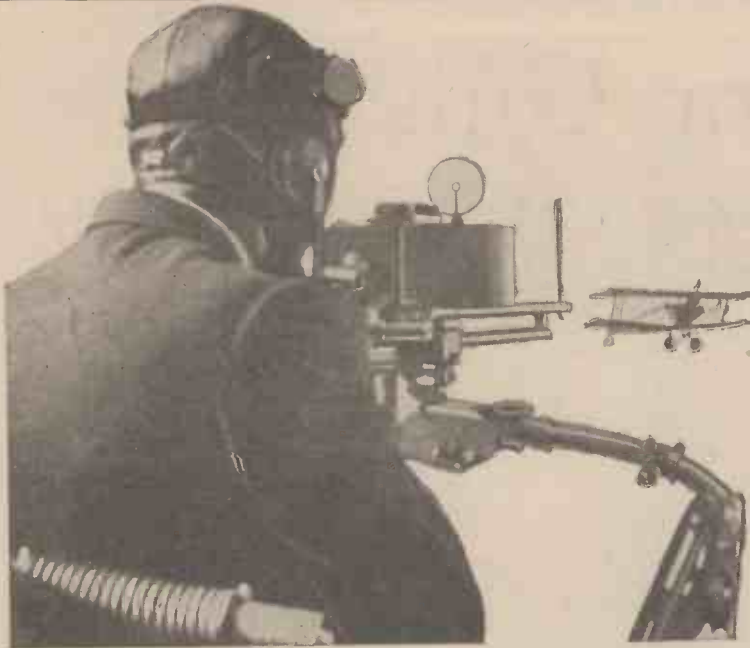
An air photographer operating a Lewis camera gun.
