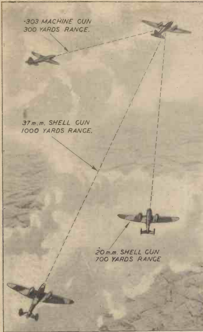
In our May issue an article in Aircraft Armament dealt with the advantages and disadvantages of machine guns and cannon. This illustration shows the effective range of each type of gun.
