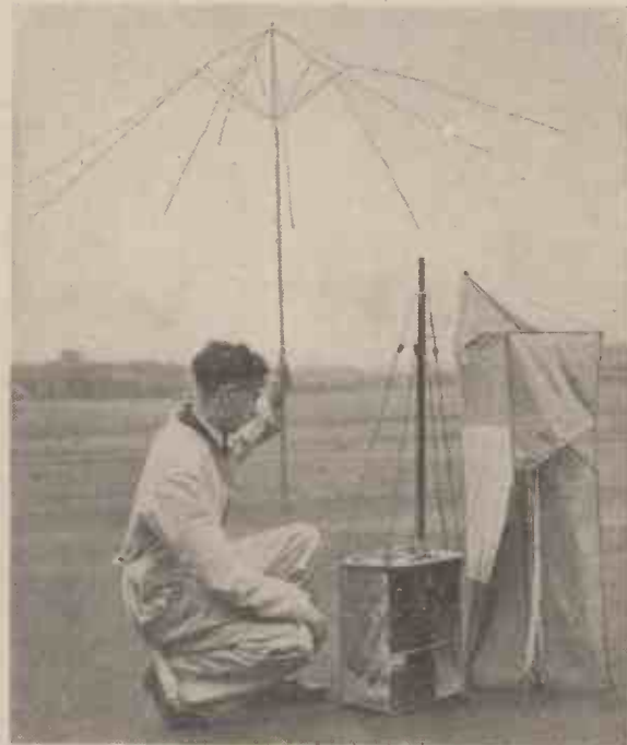
A transmitting set found in a rubber dinghy from a German bomber which crashed into the sea. It has a kite aerial, and one of the "umbrella" type. It is used to send out SOS
