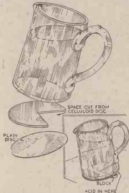
Fig. 5.—How a false bottom is formed on a jug for a simple wine and water trick
