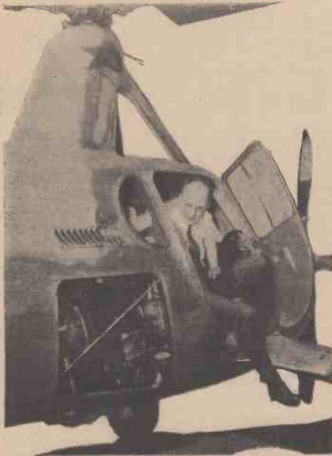
Harold F. Pitcairn, president of the Pitcairn Autogiro Corporation with his new PA-36 autogiro. Mr. Pitcairn is shown pointing out the location of the new type motor used in the 'giro. It is located in the middle of the fuselage. This gives greater visibility over the front cowling. The autogiro is capable of rising vertically, making it independent of ground obstacles or conditions of terrain. Army and navy officials inspected the craft, but have kept their findings a secret.
