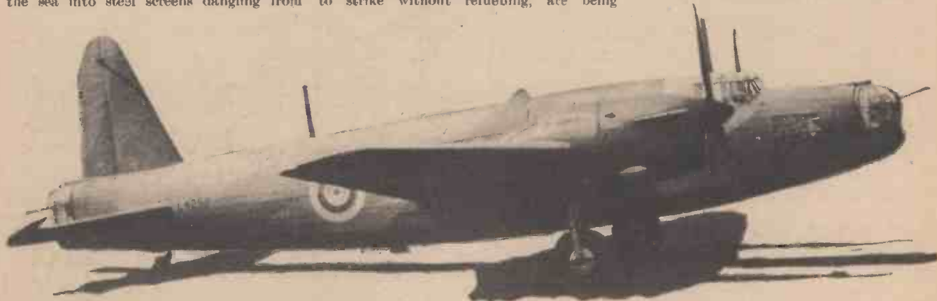
One of the famous long-range bombers of the R.A.F., the Vickers "Wellington" which has now been fitted with Rolls Royce Merlin engines.
