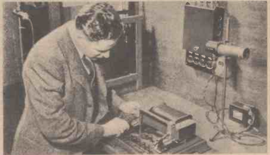
Fig. 2.—Clamping a specimen in a Fahy Simplex permeameter.
