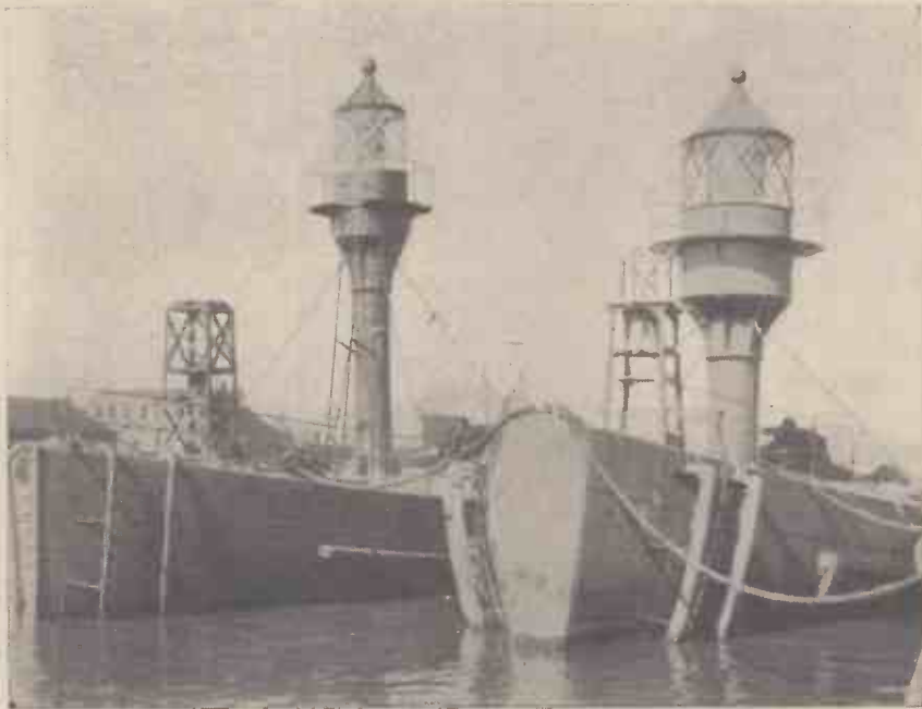
The new automatic lightships or floats which will replace the vessels which have been subjected to Nazi bombing attacks off the East Coast. The floats are automatic and need no crew. They are about 30 ft. long—half the size of an ordinary lightship—have a lantern and bell, and the lights will burn for two months unattended. To planes they would present a very small target
