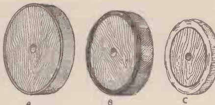
Interchangeable polishing wheels for pebble burnishing. These comprise wooden discs about 4 in. diam. and 1½ in. thick. Glued (not nailed) to the edges are: A, leather on which is subsequently glued emery grains. B, soft or chamois leather. C, silk pad or similar material
