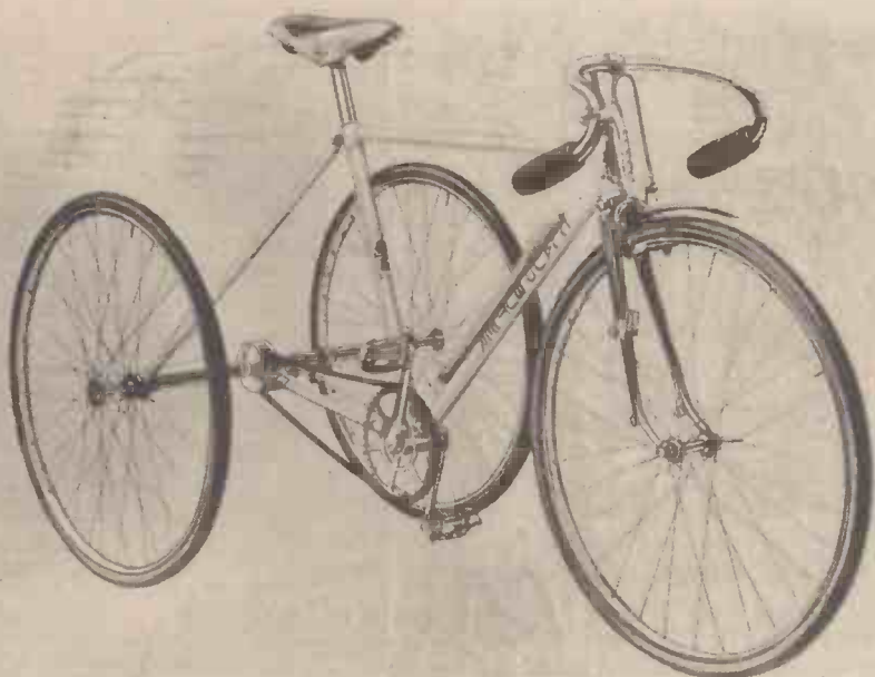
A racing tricycle of the type ridden in modern record attempts. - It is equipped with single-speed fixed gear (or freewheel), sprint wheels and tubular racing tyres. It costs 22 guineas (Claud Butler).
