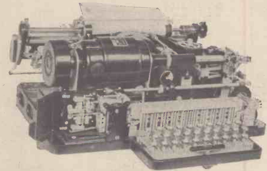
Fig. 2.—A front view of the teleprinter from the left hand side showing the transmitting mechanism.
