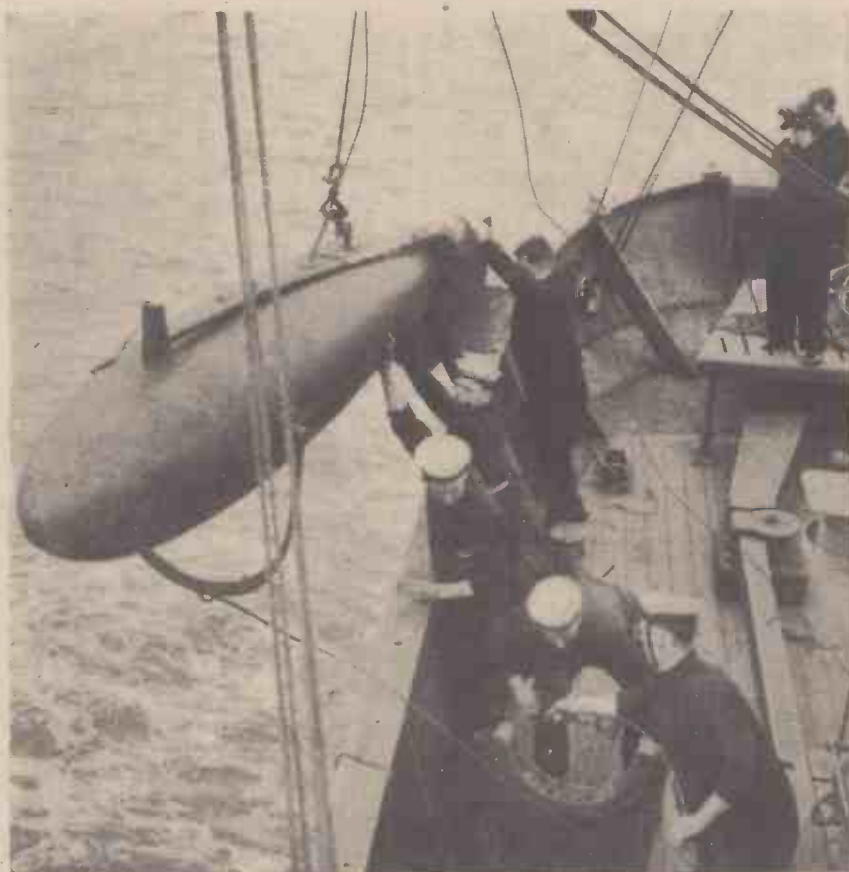
The crew on board a minesweeper lowering a paravane into the water
