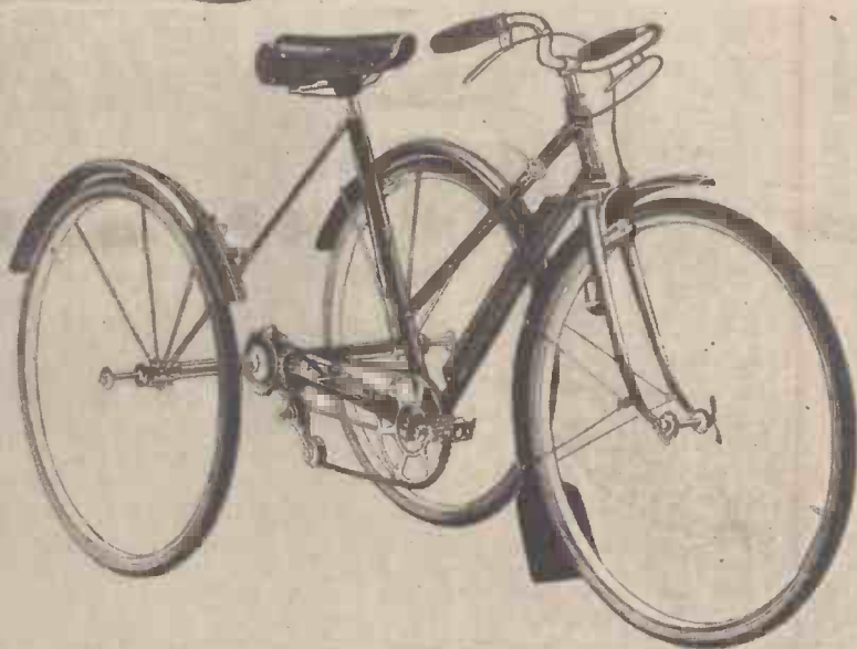
A modern lightweight touring tricycle such as is used in increasing numbers. This machine is equipped with a three-speed derailleur gear and costs 20 guineas (Claud Butler).
