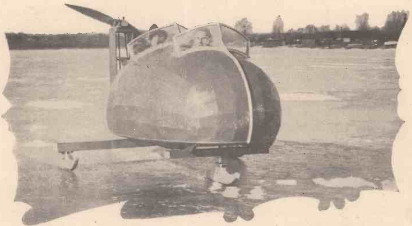
Taking an odd few moments away from the study of new designs in warplanes, tanks and the rest of civilisation's headaches, we show you the invention of Canadian sportsman Edward Rickett, of Toronto—an engine-driven sled, which from a standing start picks up a speed of 60 miles an hour or more in 200 yards. This beetle-shaped power sled can give some thrilling moments to the devotees of ice-boating—a popular winter sport in Canada
