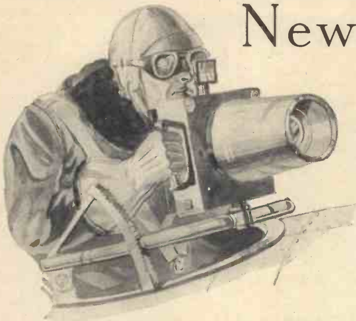
Fig. 1.—The observer of a reconnaissance plane using an aerial camera. The use of colour film is revolutionising the art of camouflage detection
