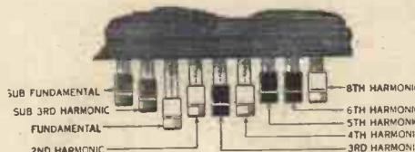
Fig. 3.—A harmonic controller. This is the device by which the artist is enabled to mix the fundamentals and any or all of eight different harmonics in various proportions
