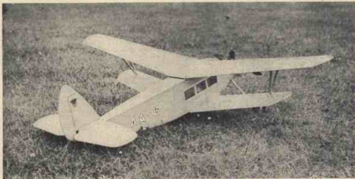
A petrol-engined biplane (9 c.c. "Brown Junior") by Messrs. J. and W. Worden, of The Model Aircraft Club
