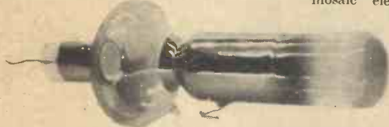
Fig. 9.—An actual example of an image-converter tube using an opaque concave shaped cathode
