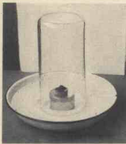
A glass jar inverted over a quantity of red phosphorus supported over a basin of water. When the phosphorus is ignited, it abstracts the oxygen from the enclosed air in the jar, leaving nitrogen
