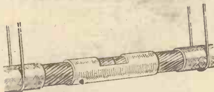
Fig. 4.—When soldering two wires together, an efficient joint can be made by using sleeving over the two ends as shown
