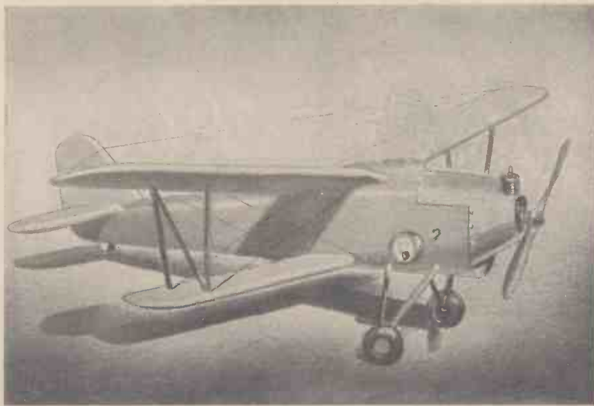
Fig. 10.—The 5-ft. biplane model which is equipped with radio control. The tuning meter which is removed for flying can be just seen above the landing gear
