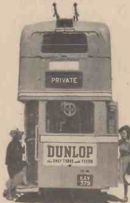
The experimental trolleybus which has been designed with a special entrance in the offside of the vehicle as well as the normal entrance. The special door is of the jack-knife type and is opened and shut by means of compressed air.
