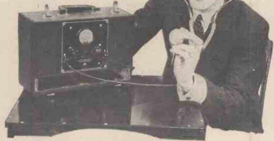
A new "loud-speaker" stethoscope, known as the Cardiophone. It is equipped with a microphone (shown in the hand of the man) which can be controlled for faint heart beats, etc., by a volume control.
