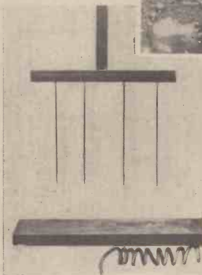
A "drop-making" machine, used for the experimental study of liquid drops.
