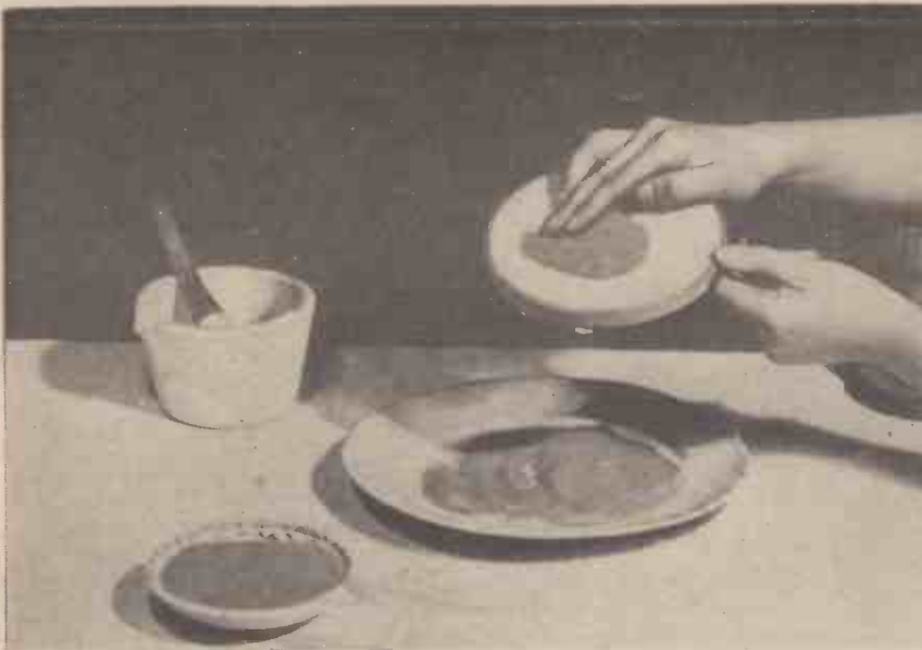
Rubbing the ground pigment through muslin in order to obtain it in the finest possible powdered form.
