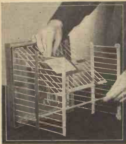
Fig. 1.—A large folding cage. The bottom slides up to the top and the sides fold inwards.
