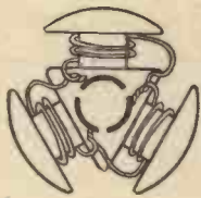
Fig. 5 (left).—How to wind the armature
